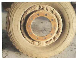
Severely dirt-contaminated wheel rim
