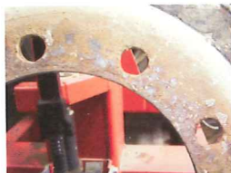
Debris trapped between wheels
