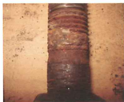
Corroded wheel stud
